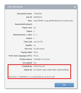
Before releasing one Job (IPPS is used for this) the Client-PC checks if he can reach the MFP by IPPS. If there are any errors an message will be displayed on the MFP display. More details can be found at the dashboard of the management.
