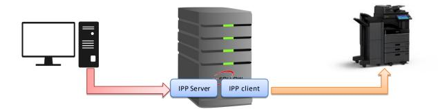
The built in IPP Server allows clients to transmit print job data via secure socket connection HTTPs/IPPs to the e-FOLLOW.cloud server. The jobs held in a virtual queue for a later release are stored fully encrypted on the e-FOLLOW.cloud server's storage.
